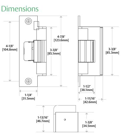
After releasing the latchbolt, the keeper returns to the locked position.
