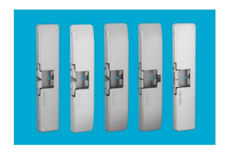
The HES 9000 series are windstorm rated, surface mounted electric strikes designed to accommodate various rim exit devices including 1/2"-3/4" throw pullman latchbolts, SecureBolt™/SquareBolt® and starwheel latches. All components are completely encased within its 3/4" thick stainless steel housing, so no cutting on the frame is required for installation.
