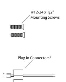
\*Only 1 Plug In Connector is used with 310-6-30
